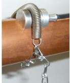
Temperature sensor with tensioning chain and spring
